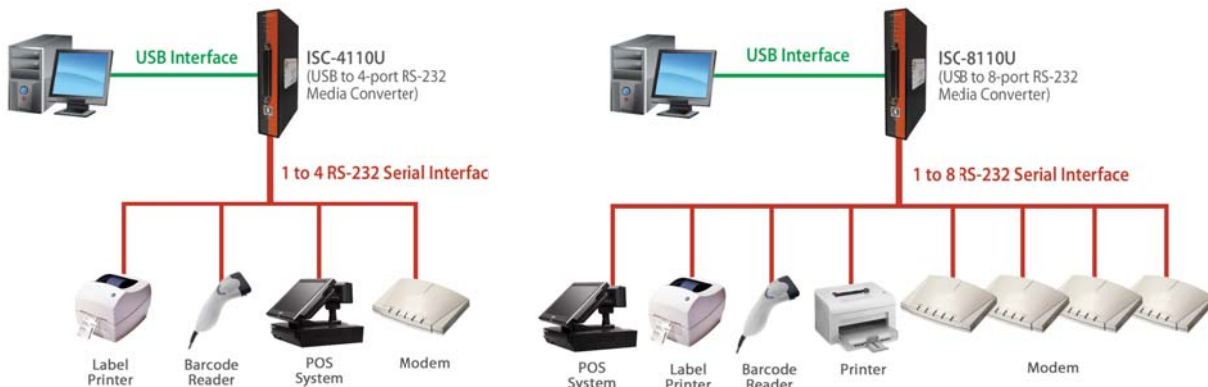
Connections of USB to Serial Media Converter
