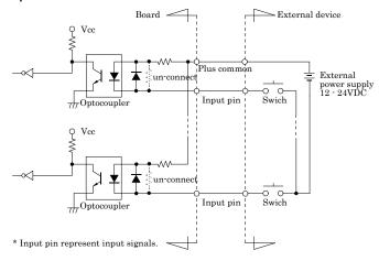
The input circuits of interface blocks of the PI-32L(PCI)H is illustrated in Figure. The signal inputs are isolated by opto-couplers (ready to accept current sinking output signals). The board therefore requires an external power supply to drive the inputs. The power requirement for each input pin is about 5.1 mA at 24 VDC (about 2.6 mA at 12 VDC).
