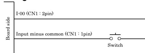
When the switch is ON, the corresponding bit contains 1.
