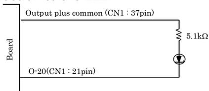
When "1" is output to a relevant bit, the corresponding LED comes on.
