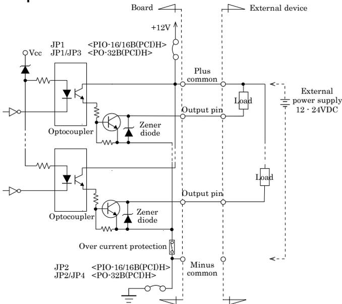
The output circuits of interface blocks of this board and PO-32B(PCI)H are illustrated in the image above. The signal output section as an Optocoupler isolated open-collector output (current sink type). To drive the output section, the on-board internal power supply must be used or an external power supply is required.
