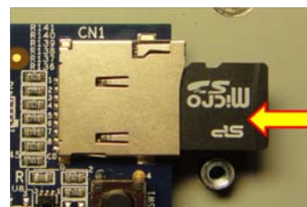
Figure 2.7-2 Insert the Micro-SD
