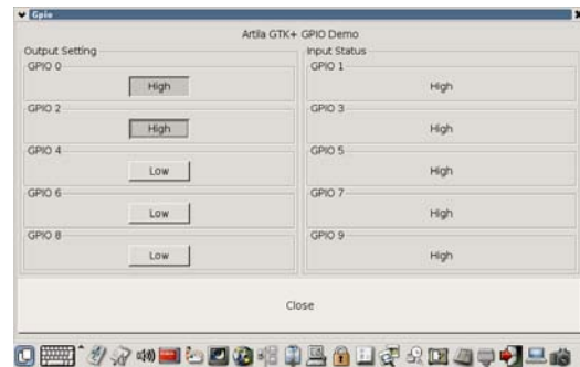
Figure 3.1.5.1-2 High of GPIO 0 ~ GPIO 3
