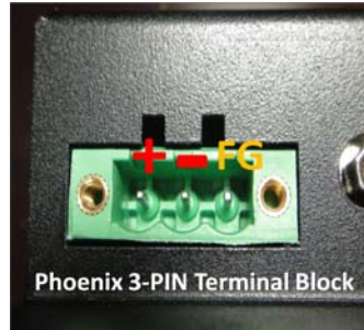
Figure 2.1-1 DC Power Input
