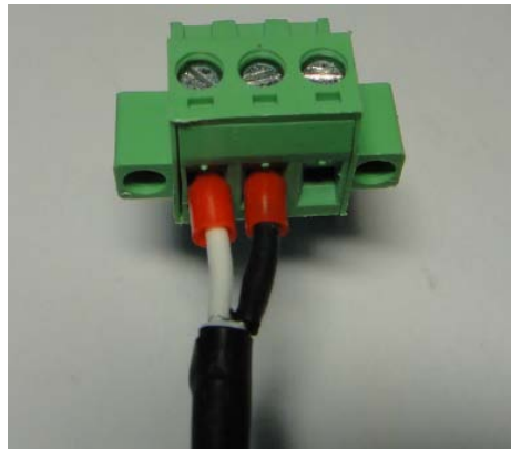
Figure 2.1-3 Plug-in with 12V ~ 40V DC Power Source
