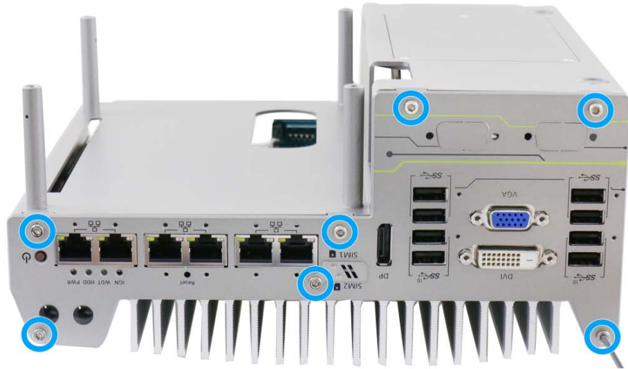
Install front panel and secure screws
