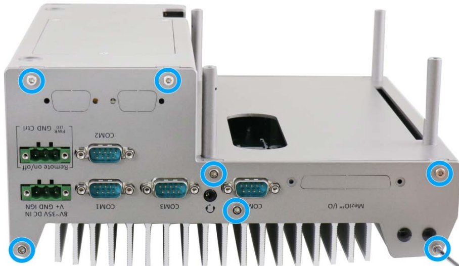
Install rear panel and secure screws
