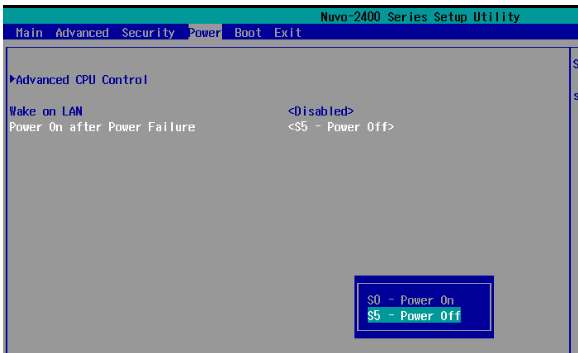
Figure 54: Configuring Power on after Power Failure in BIOS
