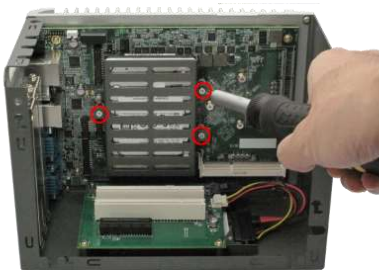
Figure 32: Installed HDD bracket assembly
