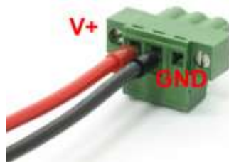
Figure 44: Wiring of DC Input Terminal Block
