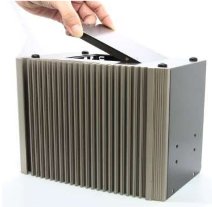
Figure 37: Wedging the HDD bracket assembly
