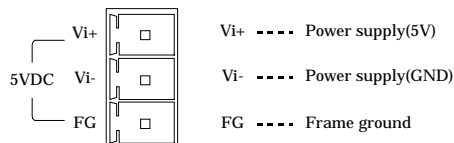
Figure 3.7. +5 VDC Input Terminal Pinouts
