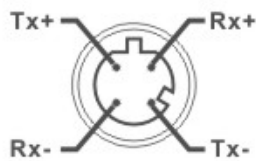
M12(4-pin, D-coding) Pin Assignments
